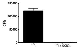
Uptake of <sup>125</sup>I by 3 x 10<sup>5</sup> cells was assayed in the presence or absence of KCIO<sub>4</sub>, an inhibitor of NIS-mediated 125 uptake.
