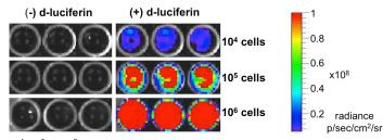
$10^4,\,10^5,\,or\,10^6$  cells were placed in wells of a 96-well plate and 0.3 mg of d-luciferin was added to the indicated wells. The plate was immediately imaged using a Xenogen IVIS Spectrum.
